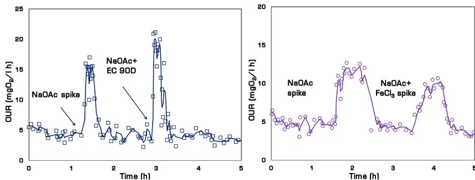
Figure 1. OUR profile of a) Ecotan Bio 90D and b)  $\text{FeCl}_3$  for the activated sludge activity inhibition estimation.
