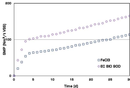
Figure 2. Potential Biomethane Production achieved from the settled sludge during the experimental trials.
